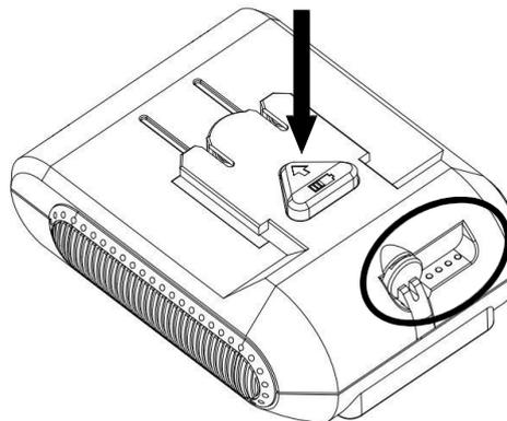
(3) Mount the battery pack onto the bottom of the sprayer.
