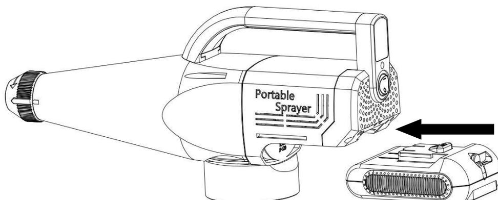
To remove the battery first lift the battery back up and then pull it out.
